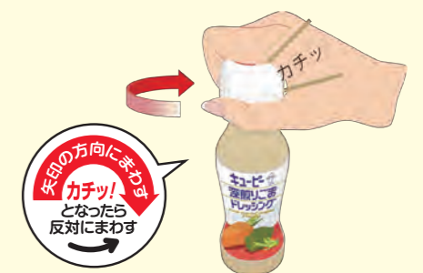
The Hineru cap opens easily, without the need to pull on the inside seal
