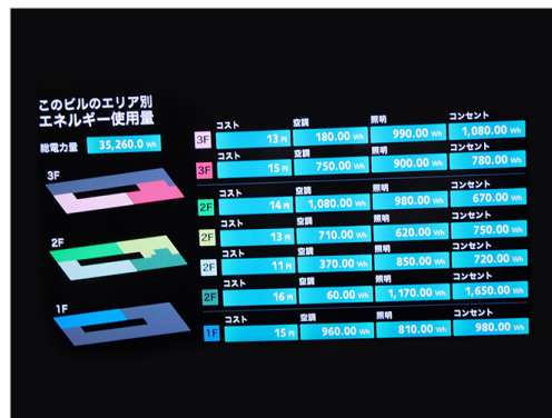
Signage displaying the amount and cost of electricity consumption by floor.
