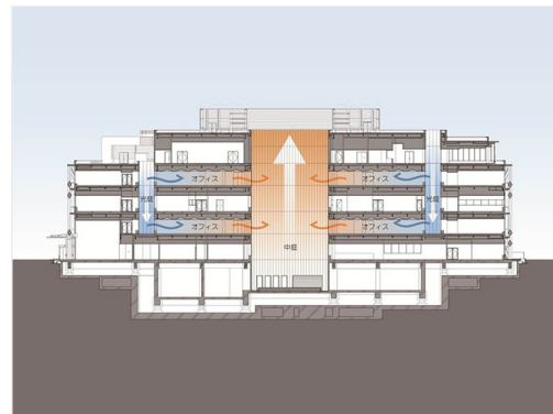
Natural ventilation system
